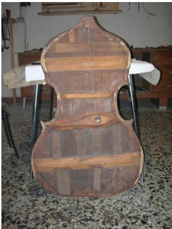
I build a wooden cross to hold the ribs on the back side as well.
