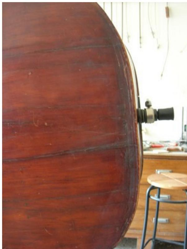
The glueing surface of the ribs to the back in this area has been lowered by 5 millimetres
