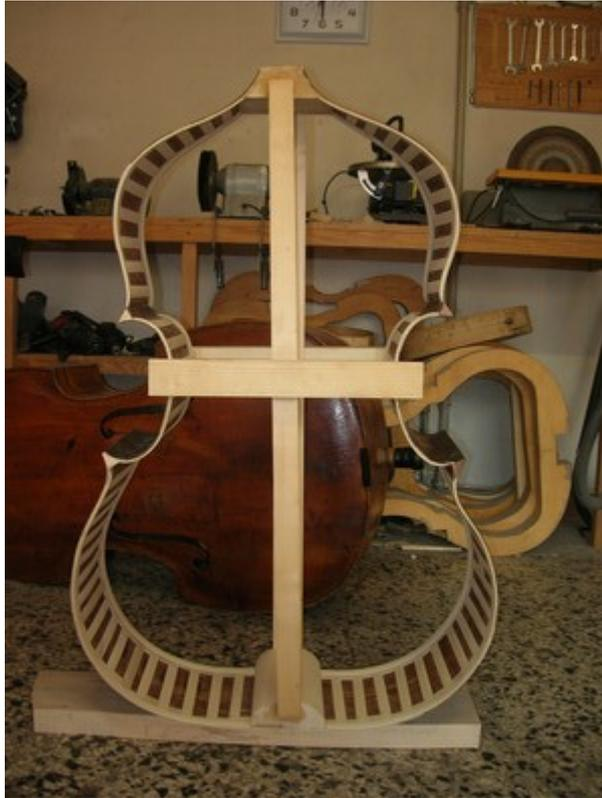
I finish the inside of the ribs, by thinning and smoothing the linings, doublings and reinforcing splints.
