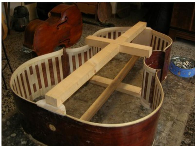
I let part of the lining on the G side lower bout jutting, where the ribs have been lowered, next to an edge replacement and where I make and glue the missing part of the rib.
