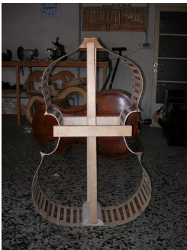
After finishing the glueing surface, I cut and glue the top linings.
