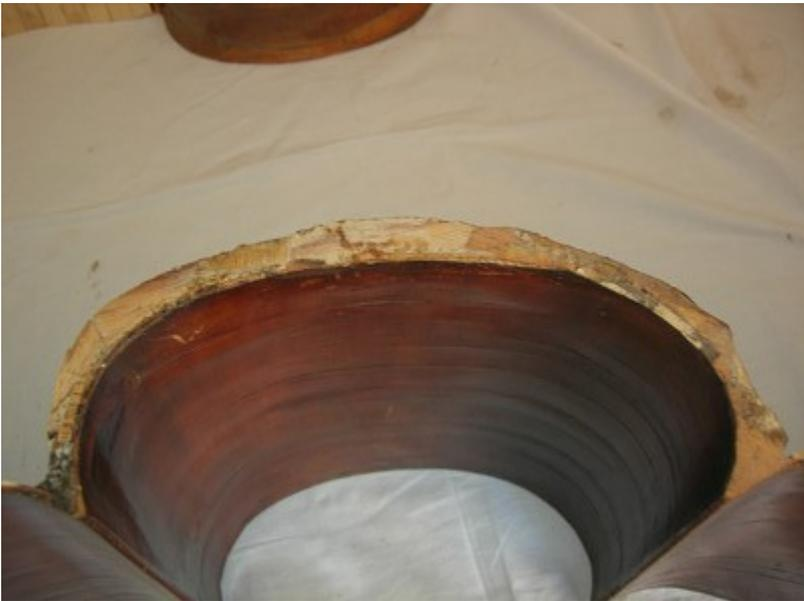
I remove the linings and reinforcements and clean the rib.
