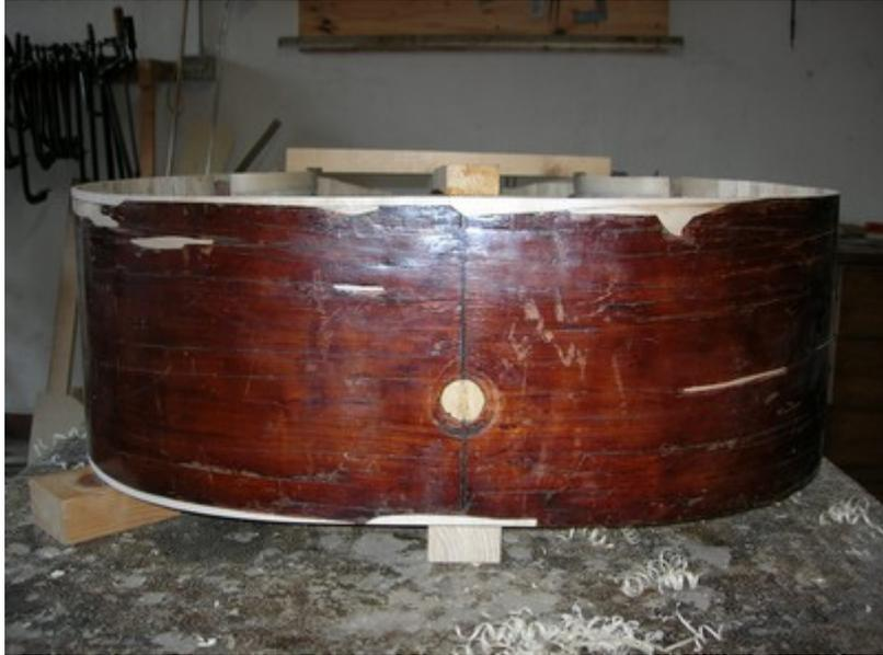
I finish the glueing surface, make and glue the linings of the back.
