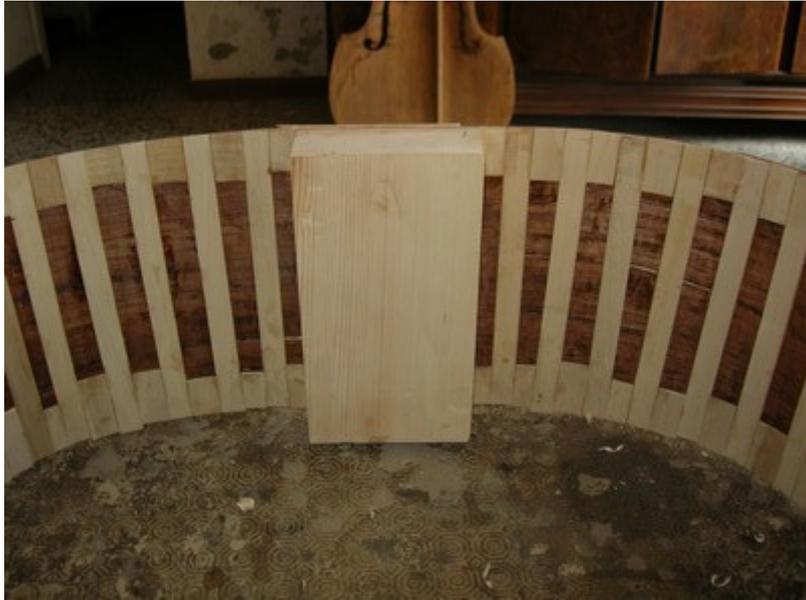
Before repositioning the crosses to keep the ribs, I start repairing the C bouts.
