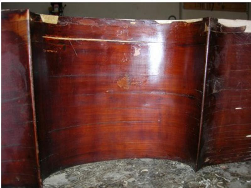
After finishing the surfaces on which the linings will be glued, I cut and bend them while verifying the shape on the top and back, and then glue them.
