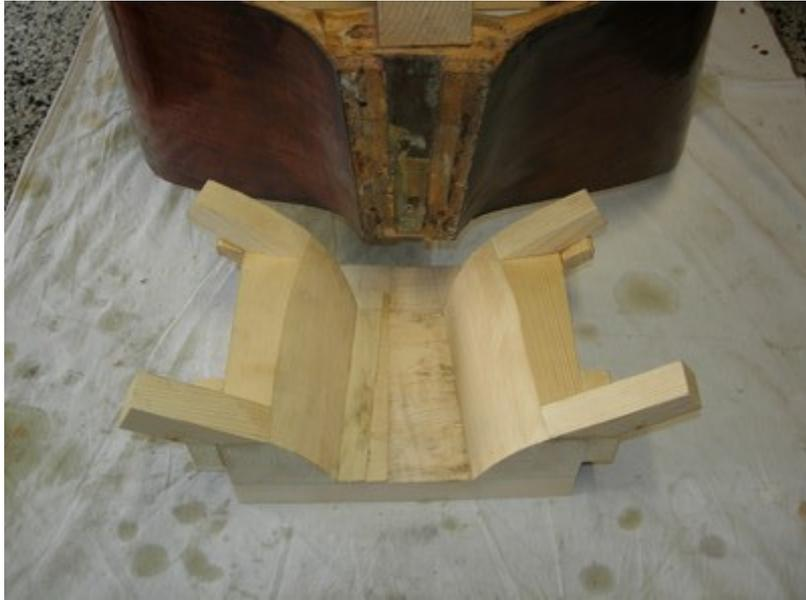
In order to remove the block, I will have to remove the wooden crosses as well.
