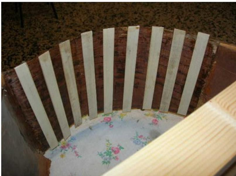
I use white maple to rebuild the missing parts and fill the shrunk cracks.
