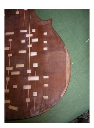
I remove the temporary cleats, clean and reinforce with new cleats.
