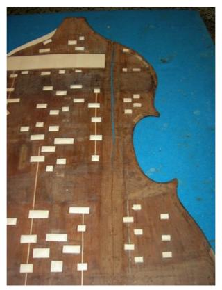
Then repair the lower part with no filling shims, replace the two upper shims and put new cleats.
