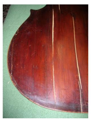
Two more cracks run parallel to the last, one between the lower edge and the glueing surface of the lower bar, the second one between the bar and the treble C bout.
