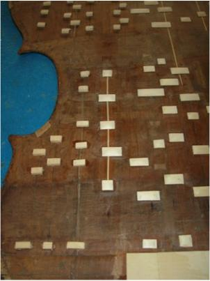
There is another open crack between the soundpost area and the lower edge, repaired with a walnut shim and putty, and two shorter cracks alongside, one right under the soundpost bar, the other at the lower edge.
