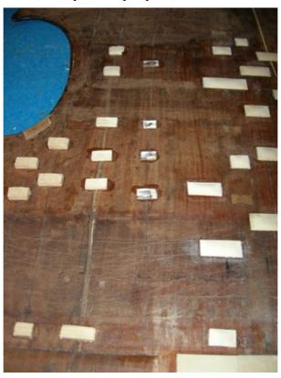
I remove the temporary cleats, clean and repair.
