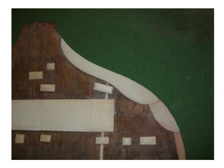
I then make an edge doubling from the bend to the lower corner, to have a better glueing surface, to secure the upper reconstruction, to thin out and make less dangerous the reconstruction at the C bout, and to fill some missing spots.
