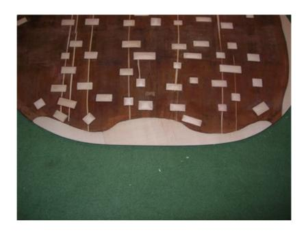
In the upper part, a crack is open from the bend to a reconstruction at the treble C bout. The reconstruction has the grain parallel to the C bout's edge.
