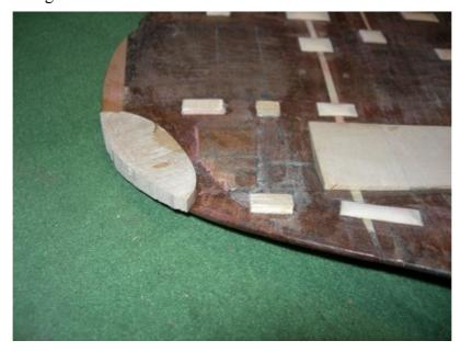
Then remove the last section of the old reinforcement at the bend.
