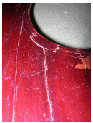
Next to this one, between the bend and the upper bar, a second small crack is open. I clean and repair the two cracks, replacing the shim with a longer one.
