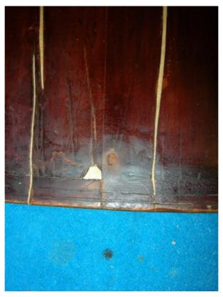
On the side of the block area there is an open crack about 16 centimetres long.
