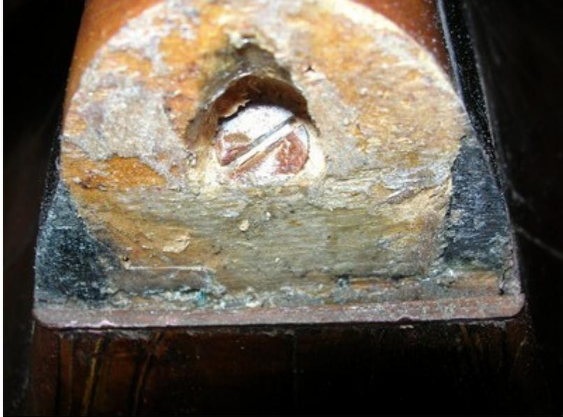
On the G side a wedge has been inserted to block the dovetailed neck fitting.
