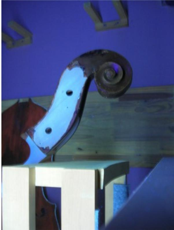
By doing so, many touches of various materials can be seen, over an homogeneous layer of varnish with gray-brownish tones.
