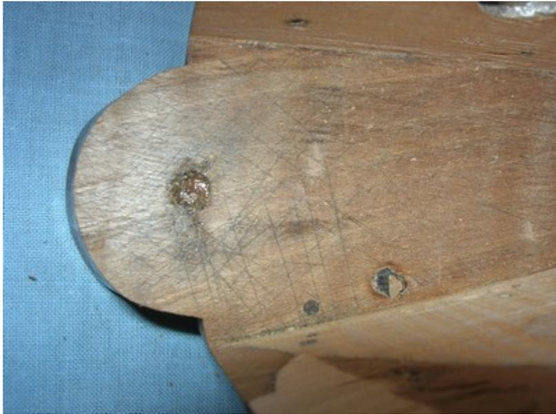
It is possible that before the last graft a screw was used for a bad repair of the base of the peg box.
