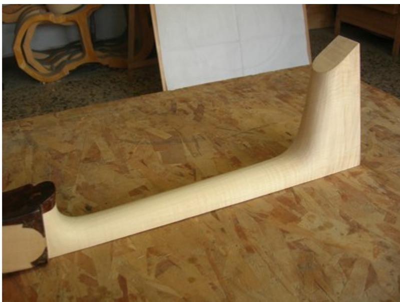
I prepare the internal part of the back button, which will be finished with an ebony crown.
