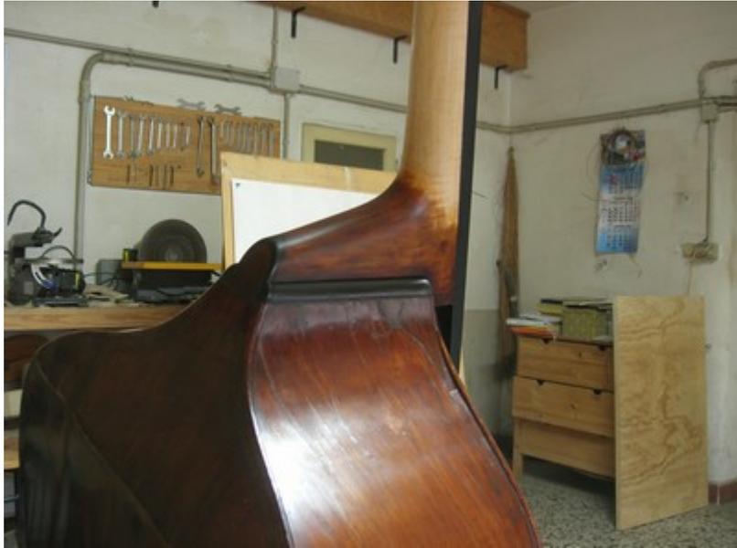
I finish the varnish on the whole instrument by French polishing, with a thin alcohol varnish, made of shellac, rosin and propolis.
