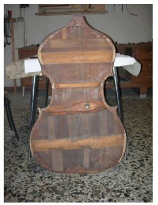
I build a wooden cross to hold the ribs on the back side as well.
