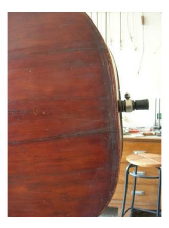
The glueing surface of the ribs to the back in this area has been lowered by 5 millimetres The endpin hole is not in the middle point of the ribs' height but more towards the top.
