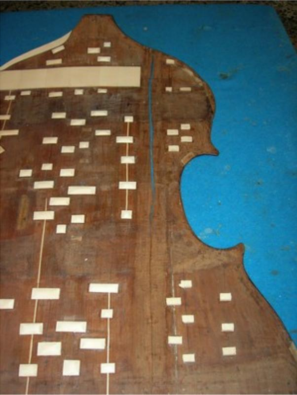
Then repair the lower part with no filling shims, replace the two upper shims and put new cleats.
