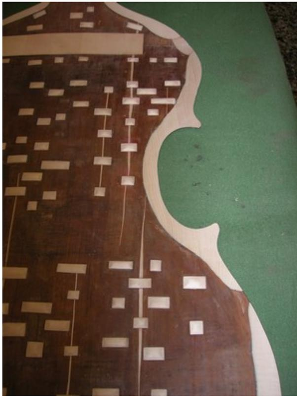
I make the last part of the reinforcement at the bend, and finish it by thinning it out.
