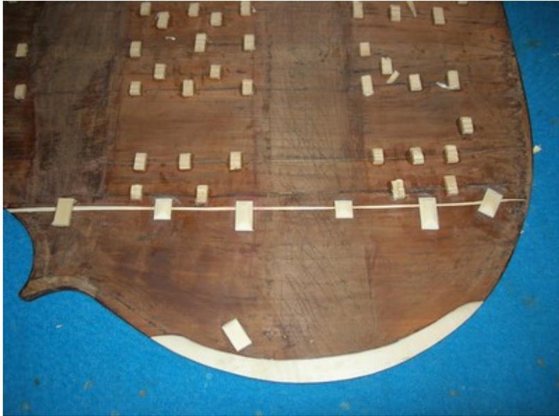
The next two cracks, above and below the lower bar, have been repaired with slivers of walnut and putty, and are partially open.
