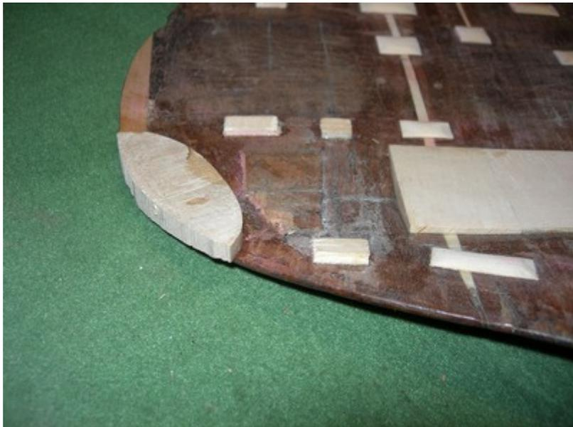
Then remove the last section of the old reinforcement at the bend.
