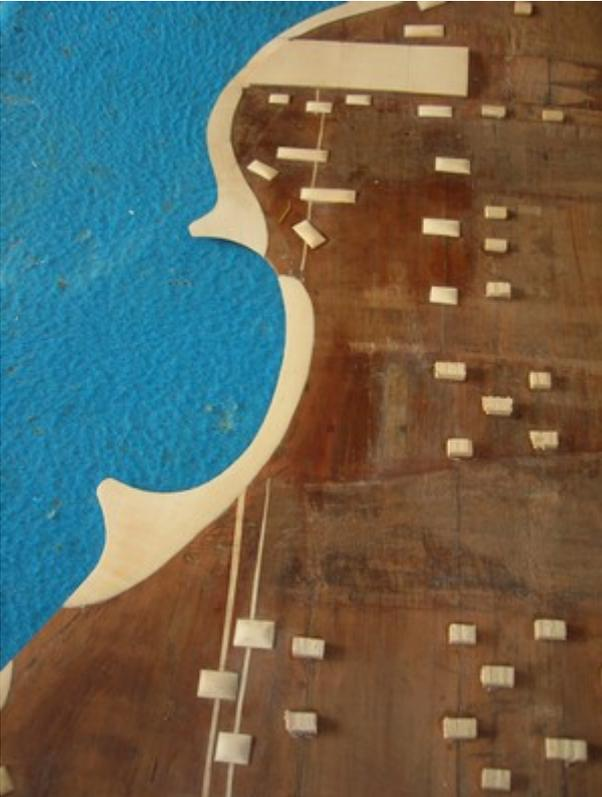
The next crack, on the lower bass side, has been repaired with a sliver of walnut.
