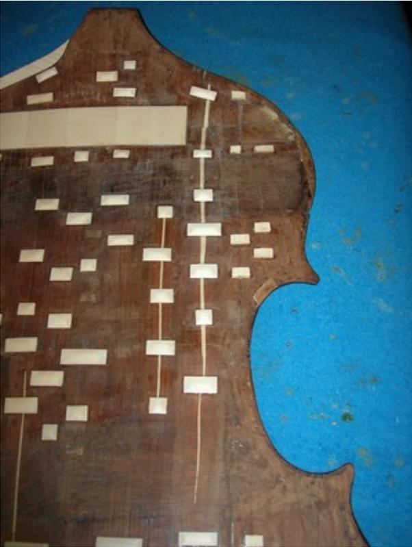
I pushed both sides of the crack on a flat surface on the outside to eliminate the sinking, while the unlevelling on the inside will remain as it is, with the cleats shaped to follow it.
