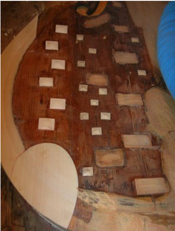
I make and insert a shim from the outside to close the first crack, which was damaged and filled.
