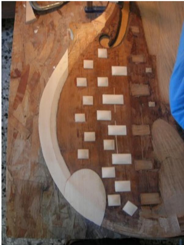
I remove a temporary cleat from the third crack and put a reinforcement under the f hole.
