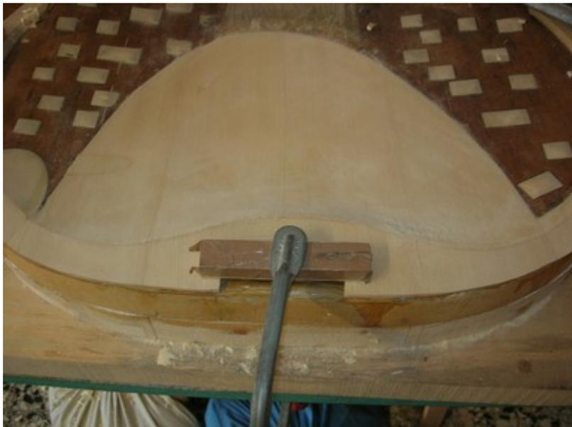
I apply a reinforcement to the lower eye of the f hole.
