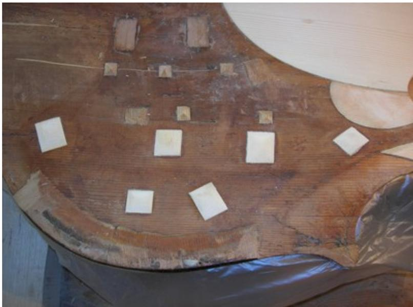
I repair the other cracks in the area that will not be covered by the upper doubling.
