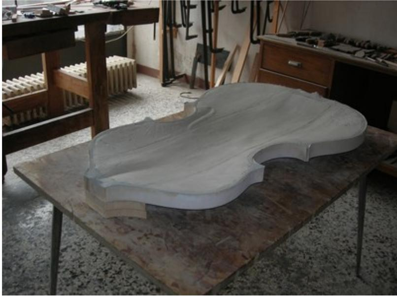
The sides of the mould are in plywood and polyester to give it strength, while the inside is in plaster for the ease to work it
