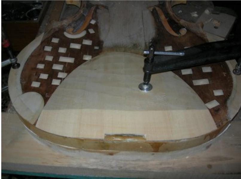
I finish by thinning and remaking the missing edge doubling, and insert a patch to get rid of a small knot.
