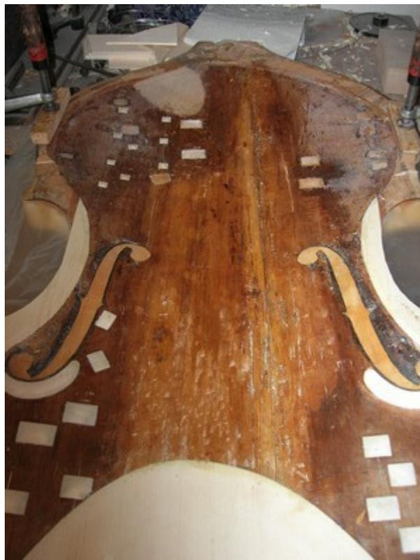
The remaining thickness of original wood varies between 3,4 and 1,7 millimetres, and is particularly thin on the bass side in proximity to the upper part of the bass bar and on the treble side on the upper part of the f hole.
