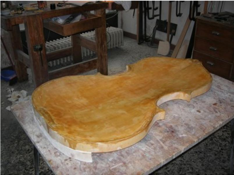
Then I press the top against the modified mould, moisturizing it and using sand bags as weights, while clamping the edges down when they rise up.
