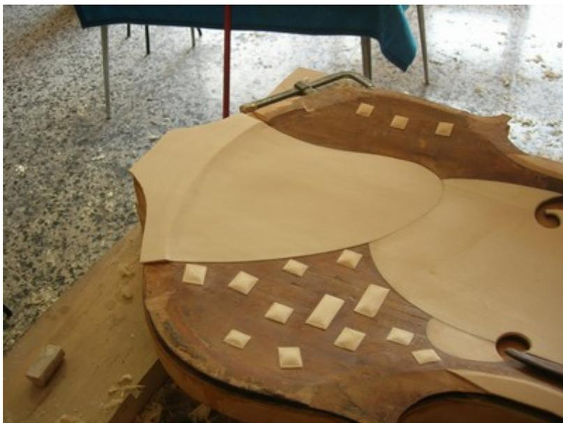
As said before, the areas next to the edge with no doubling are relatively thick, of about 5 millimetres at the upper and lower bouts, and between 7 and 8 millimetres at the C bouts.
