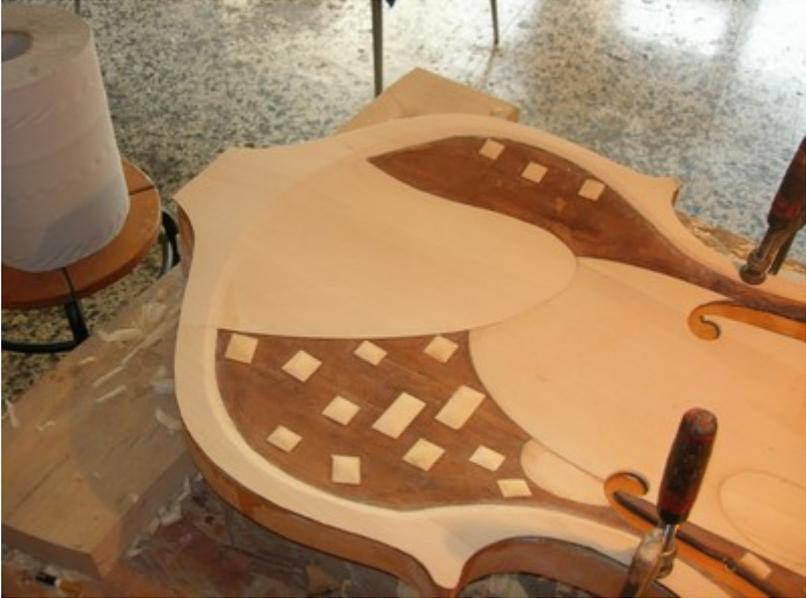
I remove the "crosses" ment to keep the ribs in shape, position the ribs on the top, trace the inside line.
