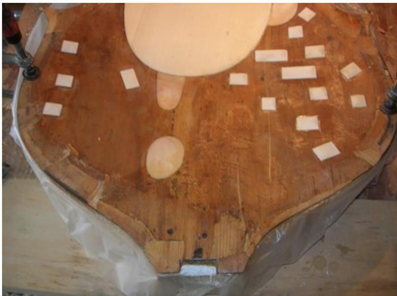
Now it is possible to see the edge reconstruction and four centering pins in the upper part of the top.
