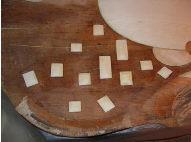
I remove the edge doubling in the upper block area.
