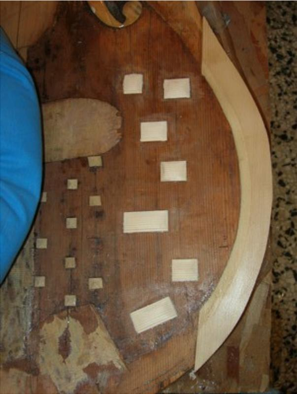
I clean the area under the edge's doubling extension towards the bass bar, to repair the inner cracks.
