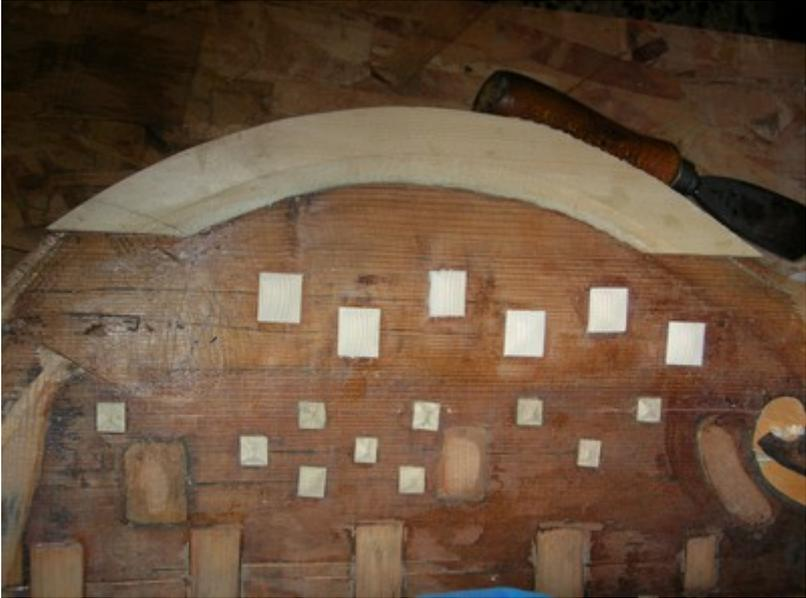
Then I replace the extension of the edge doubling, smoothing the edges thus obtaining a curve glueing surface.
