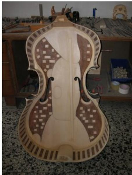
I set a splint between the C bouts on the back side to hold the correct width.
