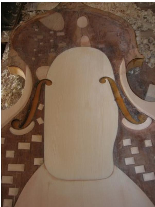
In order to avoid stiffening this part too much, considering the inclined fiber and the large glueing surface, I use softer spruce than the one used in the lower part.
