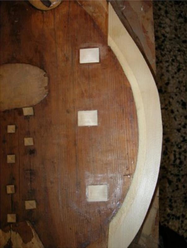
I clean and repair the other cracks, always reinforcing with new cleats.
